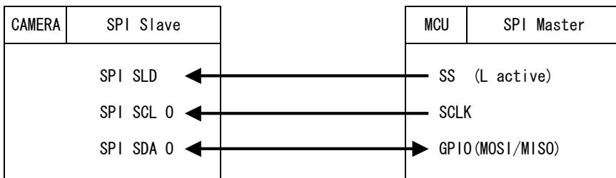
Both directions (input and output) are required for GPIO of external MCU (master), and in order to do bidirectional communication (MISO/MOSI), it needs to be switched direction (input or output).
